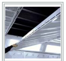
Hinged ceiling filter frames for easy replacement of 10 micron media filters.
